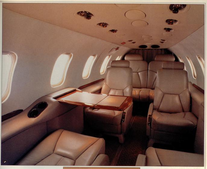
this is no stripped-down airplane. To the right is the newly redesigned cabin interior with seating for seven to eight, depending upon configuration. One of the new options is an aft lavatory, though the airplane we photographed was equipped with a lav opposite the cabin door.
